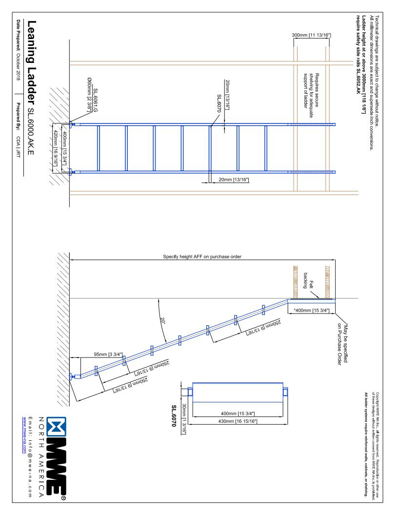
Ladder height at or above 3000mm [118 1/8"] require safety side rails SL.6052.AK Technical drawings are subject to change without notice.
