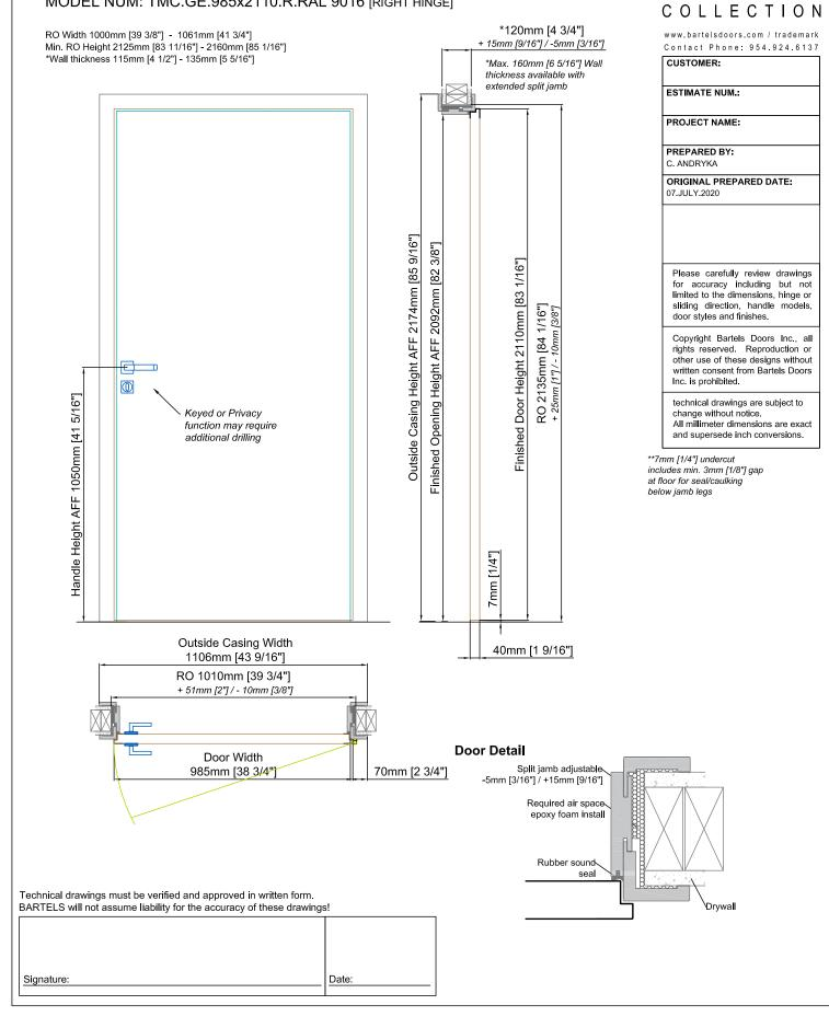
MODEL NUM: TMC.GE.985x2360.L.RAL 9016 [LEFT HINGE]
