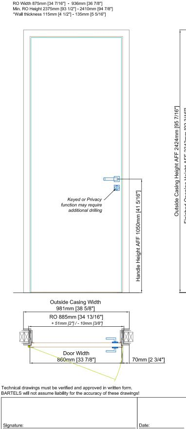
\*120mm [4 3/4"] + 15mm [9/16"] / -5mm [3/16"] \*Max. 160mm [6 5/16"] Wall extended split jamb Finished Opening Height AFF 2342mm [92 3/16"] Finished Door Height 2360mm [92 15/16"] RO 2385mm [93 7/8"] + 25mm [1"]/ - 10mm [3/8"] 7mm
